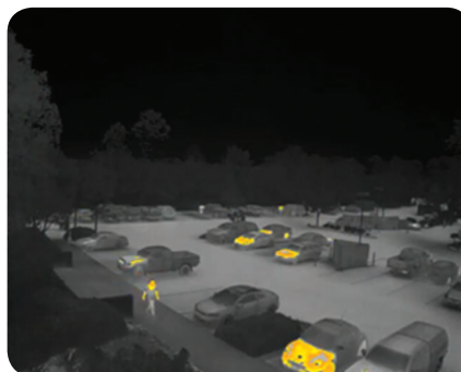
Manually set isotherm thresholds to colorize temperatures of interest (mid-range) in the grey scale
